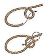
The Bowline is an ancient knot which is very strong. It used to form a fixed loop which doesn't slip at the end of a rope.
